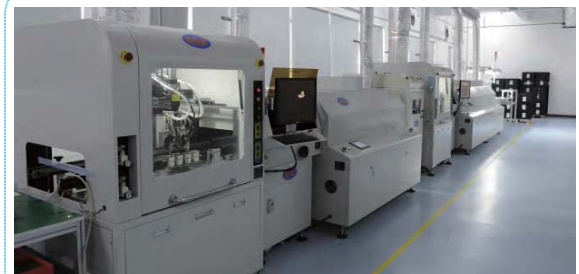
Note: The automatic spraying process of conformal coatings
